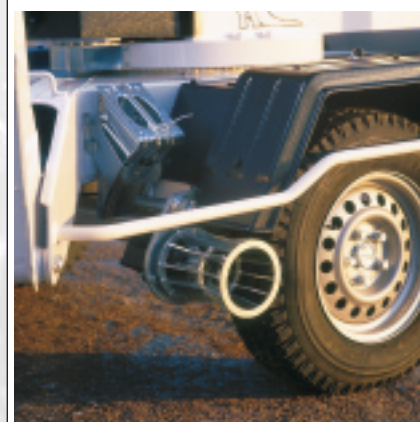
DINO drive system provides easy positioning on job site.
