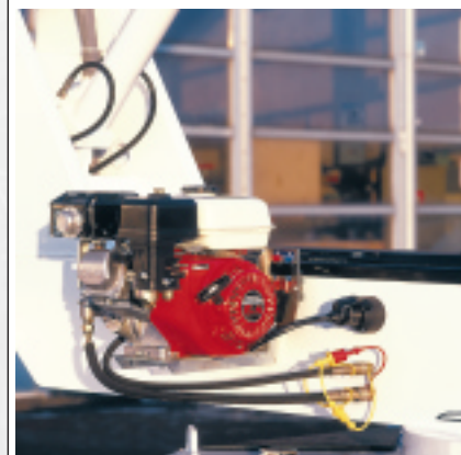
Optional gas engine features quick couplings to provide additional power source.
