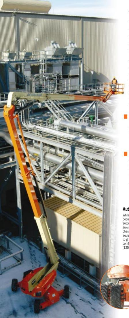
The all-new JLG Model 1250AJP articulating boom lift delivers the additional reach capabilities only an articulating boom can provide for applications that demand more flexibility.
