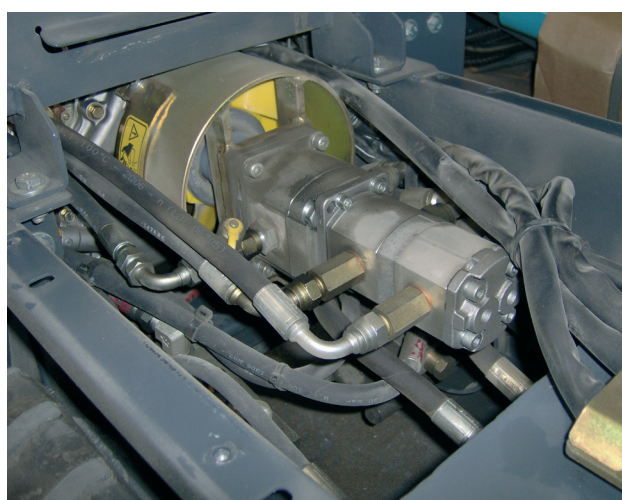
Detail of the Hydraulic oil cooling system (Patented) Detail Kühlsystem Hydrauliköl (Patentiert)
