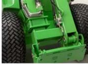
Hydraulic quick attachment coupling plate
